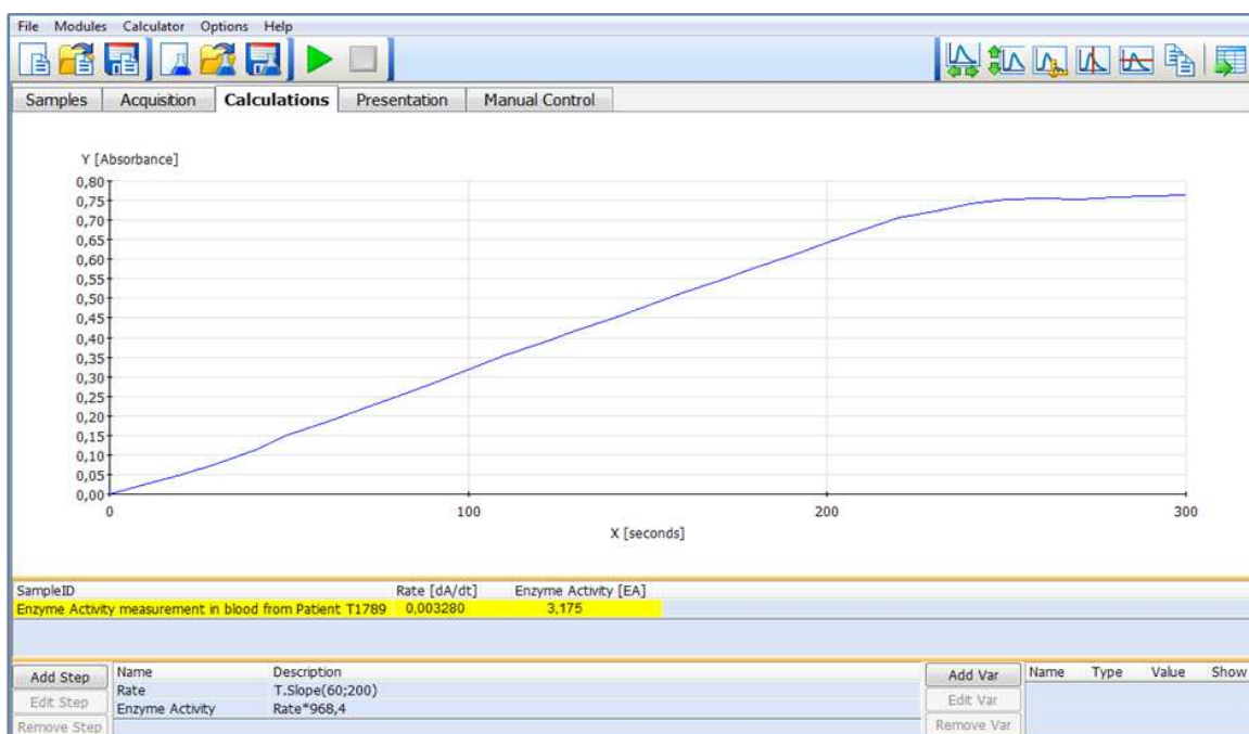
Figure 10: Typical Enzyme kinetics graph, showing the increase of absorbance over time. This graph is shown in the "Calculations" tab of the Timedrive method for enzyme activity determination. The experiment was carried out over 5 minutes (300 seconds) and the absorbance increased from 0.0A to approximately 0.7A. To obtain the desired result, two simple calculations are applied: In the first step the slope of the curve is determined. As the curve has some non-linear portions, the slope is only calculated in the range between 60 and 200 seconds. In the second step, the slope (rate) value is multiplied with an enzyme-specific factor (in this example it is 968,4) to give the result (=Enzyme Activity) of the single sample measured in this example.
